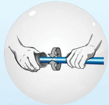
Chamfer the external edge of the pipe to make it easier to fit into the fitting and to avoid damage to the seal. Chamfer the inner edge eliminate any cutting residues.
