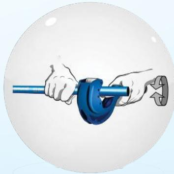
The pipe must be cut perpendicular to its length (ref. PPS CTU).
