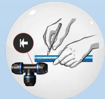
Mark the tube to indicate the insertion depth in the fitting (use the reference marks on the fittings or on the wrench).
