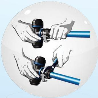
Re-screw the nut by hand, and then tighten according to recommendations.
